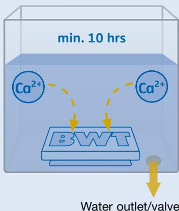
Change the bestsave limescale protection pad as soon as the maximum number of units (number of tank refills) have been reached. You can work out the potential number of refills quite easily by using the table below. Just match your local limescale content (water hardness) with the size of the water tank used and read off the number of refills – job done.
